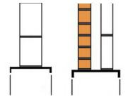
Where the external face of the wall is at or near to the edge of the foundation block, it is sufficient to ensure that the vertical centre line of the wall is within the middle third of the foundation width.
